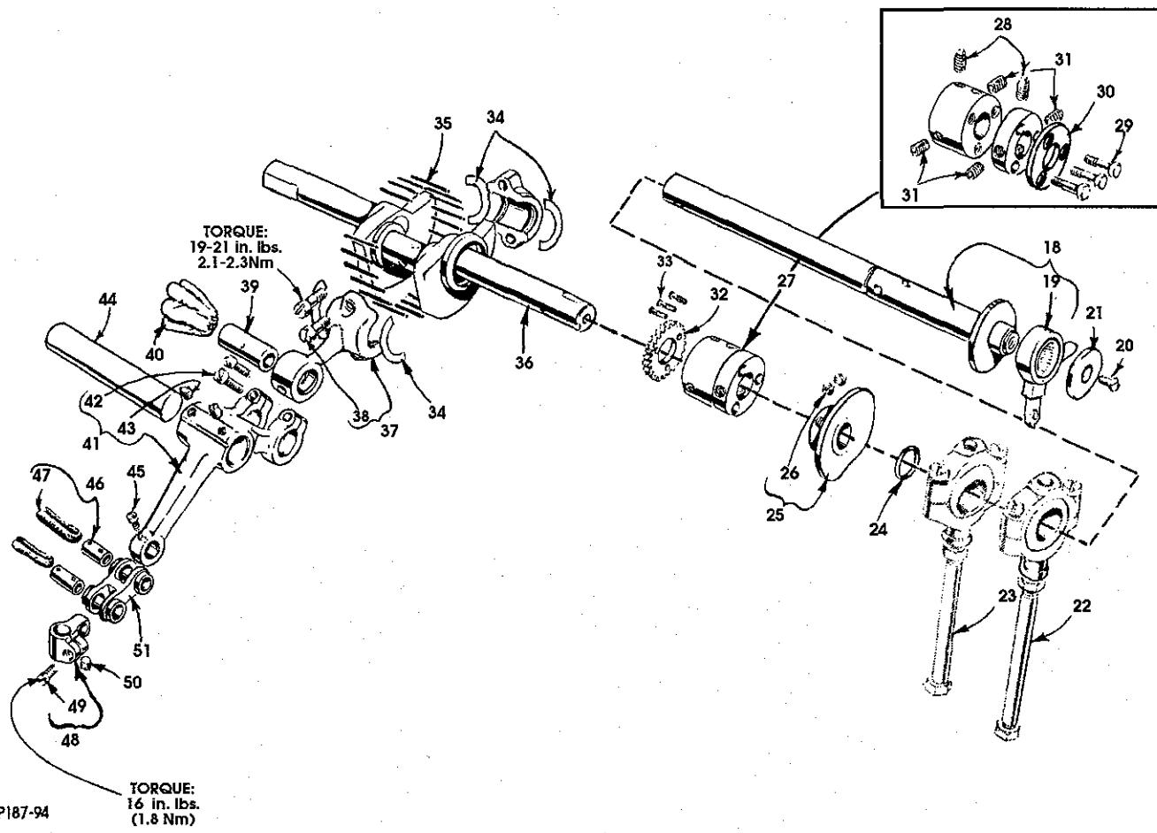
**MISCELLANEOUS OILING, NEEDLE LEVER, CRANKSHAFT AND MAIN SHAFT PARTS
