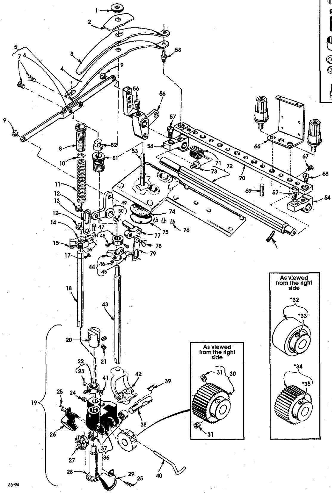
**UPPER ROLLER FEED, FOOT LIFTER AND THREAD TENSION PARTS (CONT.)**
