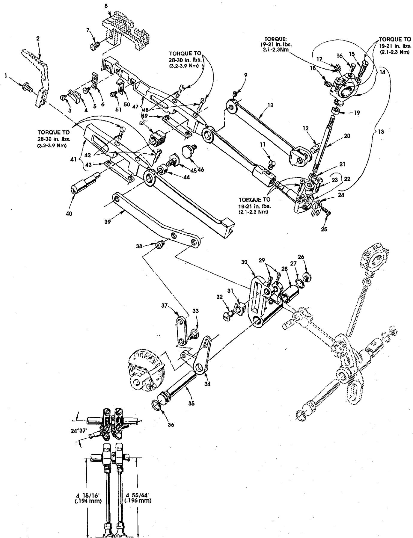
**DIFFERENTIAL FEED BAR, MAIN FEED BAR, FEED LIFT ECCENTRIC ASSEMBLY
